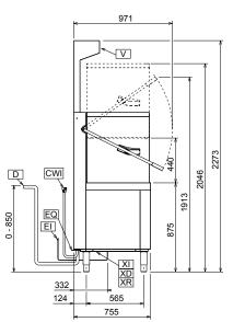
Cold Water inlet 1 (cleaning) D Drain
